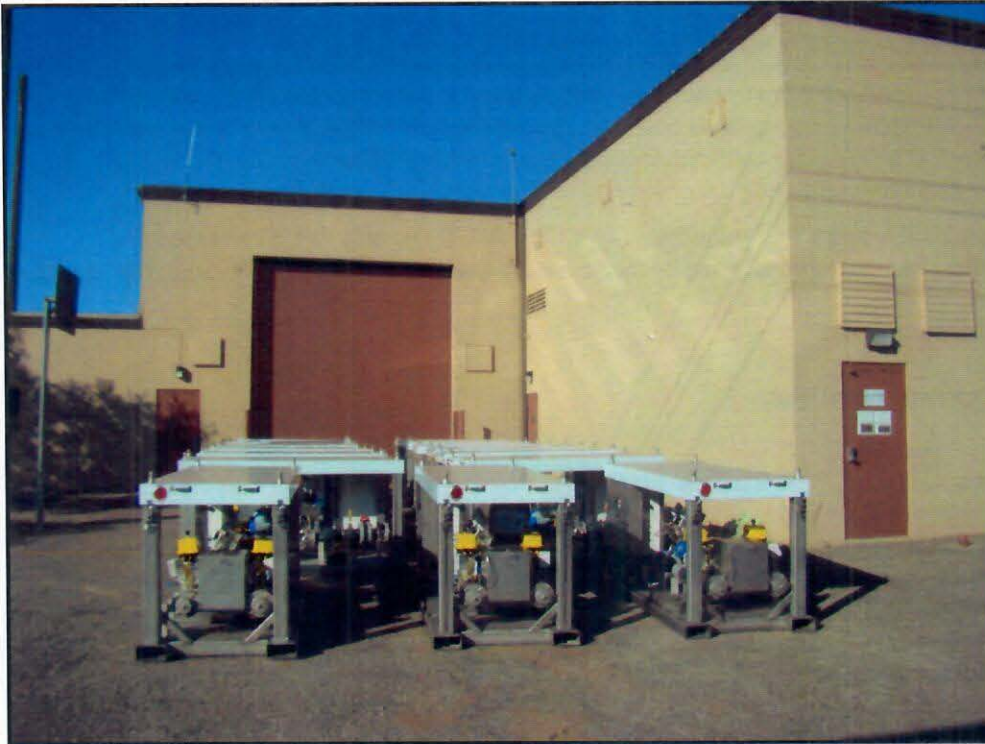
Figure 6. Remote Valves Used for Rainfield Modifications.
